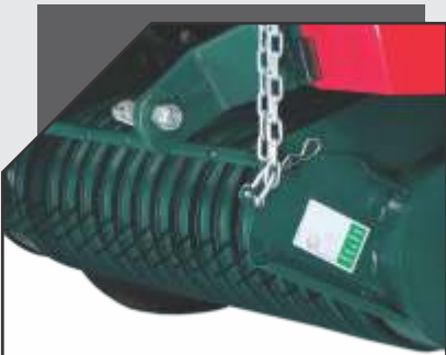
GRADE 3 SPRING STEEL FOR REEL TINES
