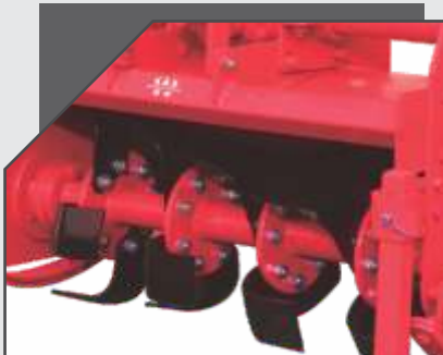
BORON STEEL BLADES WITH HELICAL ROTOR DESIGN
