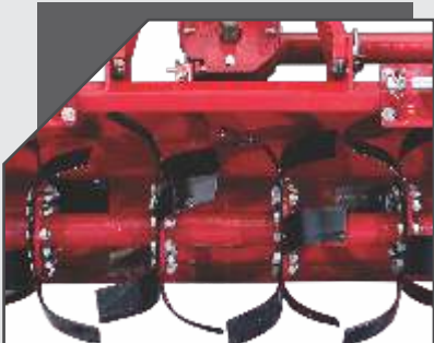
BORON STEEL WEAR RESISTANT BLADES
